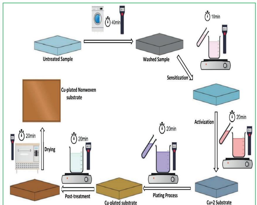
Figure 1. Schematic illustration of the process of laser-treated conductive Nonwoven via electroless deposition
