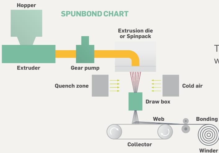
The two outer layers are made with the **nonwoven spunbond process**.
