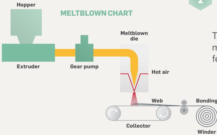
The middle layer in a medical mask is made with a **nonwoven meltblown process** featuring electrostatic charging.
